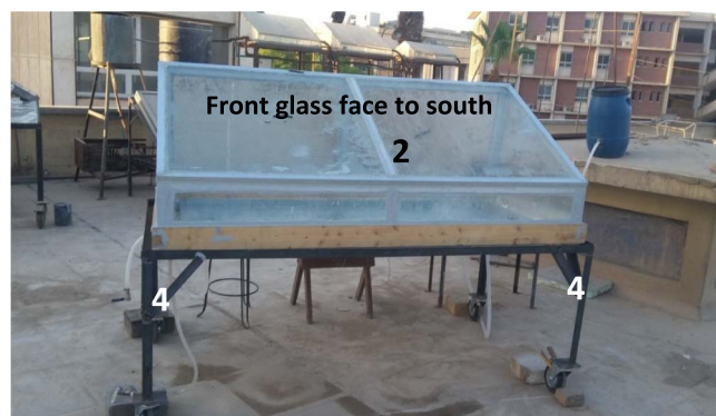
Fig. 1. Front view of the solar still.
