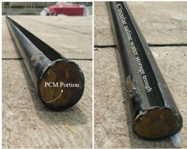
Fig. 2. Circular water storage trough with PCM.
