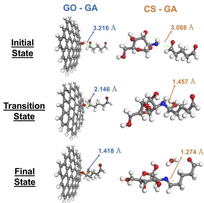
Fig. 2. The mechanisms of the two cross-linking processes. (gray atom: carbon, white atom: hydrogen, red atom: oxygen, blue atom: nitrogen). (For interpretation of the references to color in this figure legend, the reader is referred to the web version of this article.)
