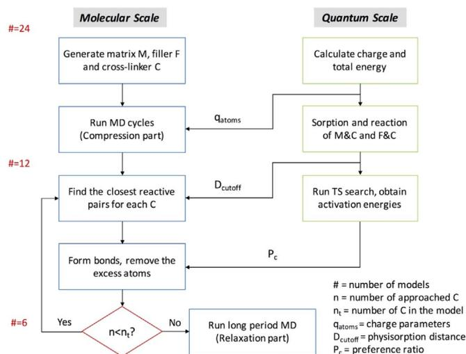
Fig. 1. Modeling scheme used in this study combined with molecular and quantum scale.
