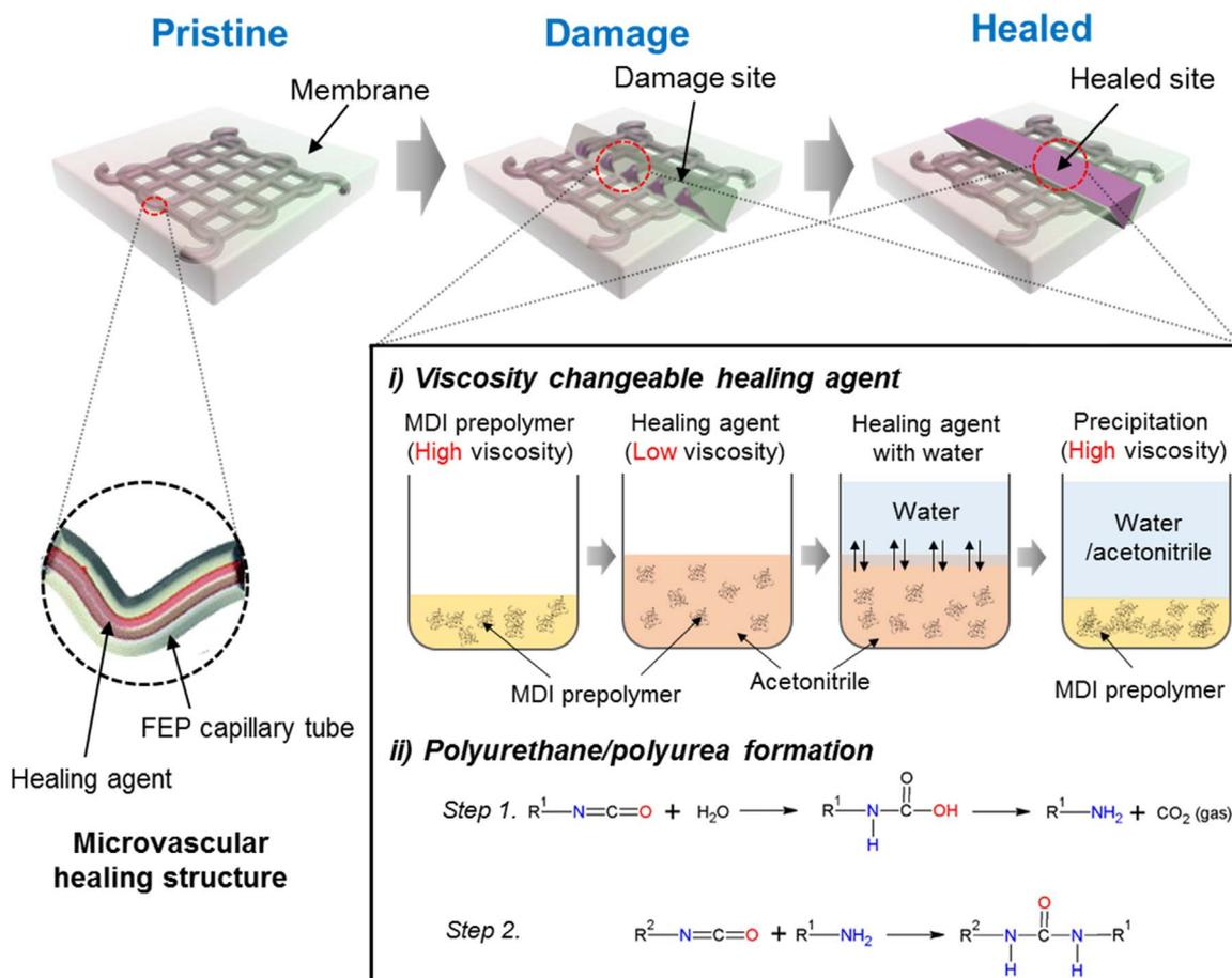
**Fig. 1.** Structure of a microvascular network-embedded self-healing membrane and schematic illustration of the healing mechanism. When the membrane structure is physically damaged, the microvascular network releases a reactive healing agent. Upon contact with water, the healing agent precipitates into a viscous prepolymer that further rapidly reacts with water to form a polyurethane/polyurea matrix that fills the damaged site.
