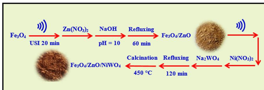
**Scheme 1.** Schematic illustration for the preparation of  $\text{Fe}_3\text{O}_4/\text{ZnO}/\text{NiWO}_4$  nanocomposites.
