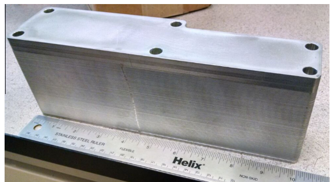
Fig. 1. Overall design of the micro-channel heat exchanger for this work.
