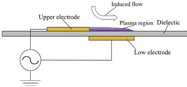
Fig. 1. Schematic diagram of a normal DBD-PA [1–6].
