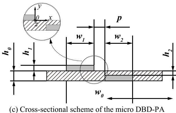
(c) Cross-sectional scheme of the micro DBD-PA
