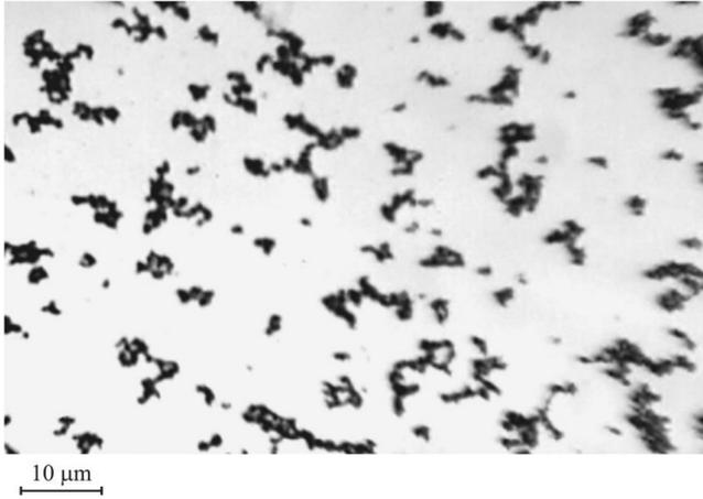
**Fig. 1.** Microphotography of magnetized aggregates typical of vacuum oil (VO-3)-based magnetic fluids.
