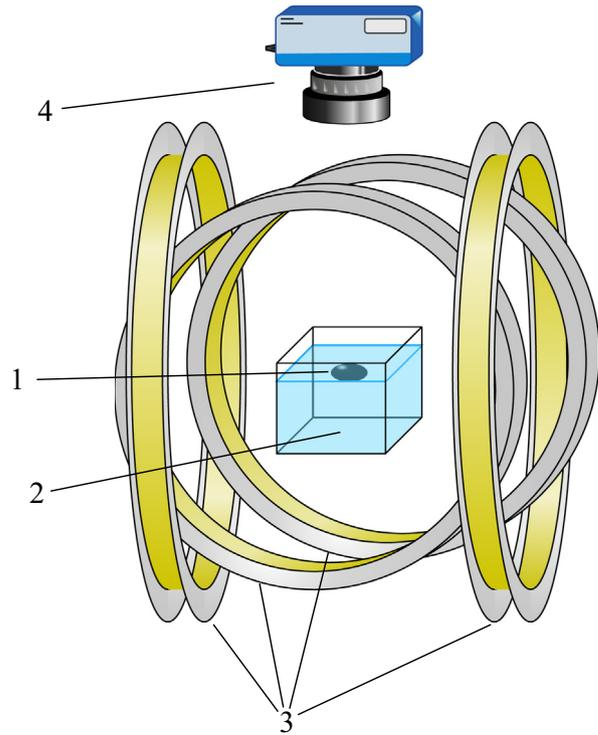
**Fig. 3.** Schematic of the experimental setup used to investigate the behavior of the drop on the water surface: 1 – MF drop, 2 – water-filled cell, 3 – two crossed pairs of Helmholtz coils; 4 – video camera.
