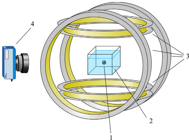
**Fig. 2.** Schematic of the experimental setup used to investigate the falling of an MF drop: 1 – MF drop, 2 – water-filled cell, 3 – two crossed pairs of Helmholtz coils; 4 – video camera.
