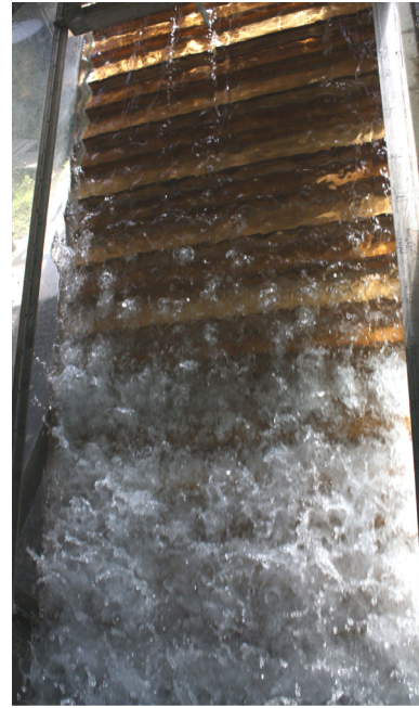
(B) Laboratory scale: Present study, h = 0.05 m, \theta = 26.6^\circ , d_c/h = 2.22 , q = 0.116 m 2 /s, Re = 4.6 \times 10^5 (Flow from top to bottom)
