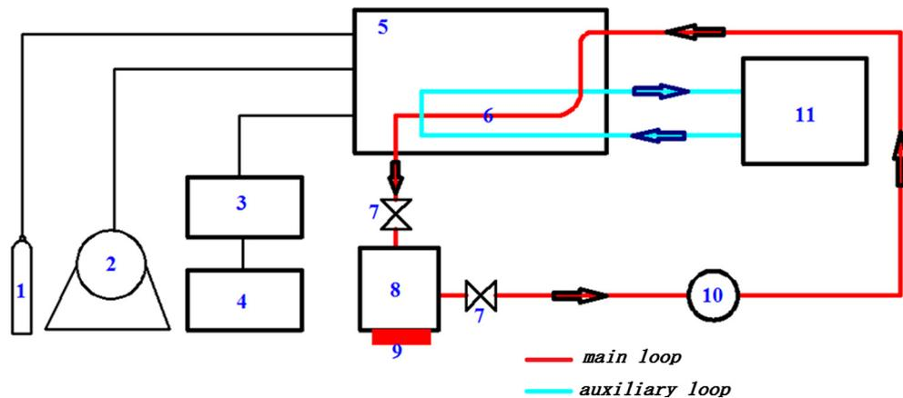
Fig. 1. Schematic of experimental system: 1 argon; 2 vacuum pump; 3 Agilent data-acquisition instrument; 4 computer; 5 test section; 6 test sample; 7 valve; 8 storage tank; 9 copper heating block; 10 peristaltic pump; 11 thermostatic water tank.
