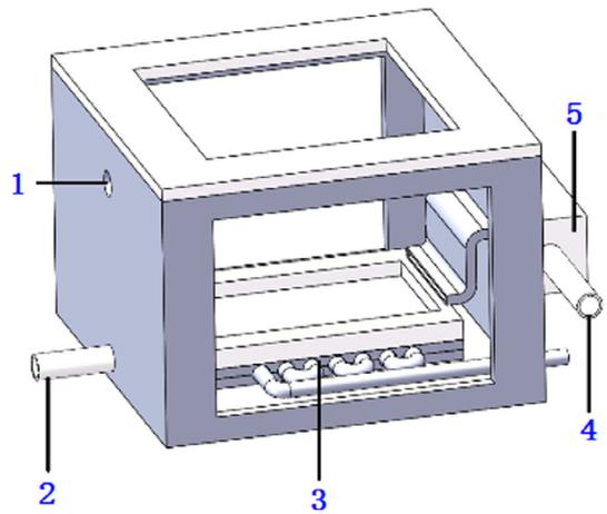
Fig. 2. Schematic of the test section: 1 vacuum-argon system; 2 temperature monitoring point of outgoing liquid metal; 3 test sample; 4 temperature monitoring point of incoming liquid metal; 5 buffer tank for liquid metal.
