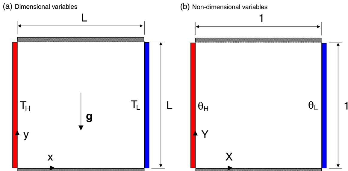
Fig. 1. Physical model of the square cavity for natural convection.
