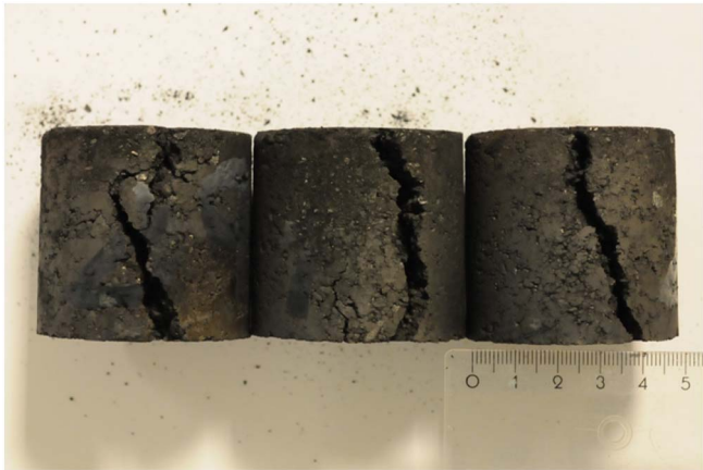
Fig. 1. Samples of ramming paste which have cracked during baking. Source: Elkem Carbon.
