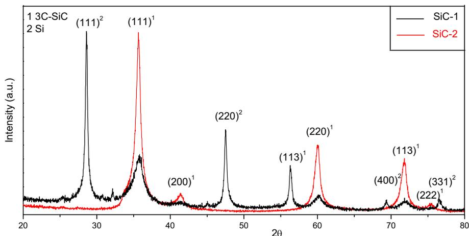
Fig. 1. Superposed X ray pattern for the SiC-1 and SiC-2 powders.
