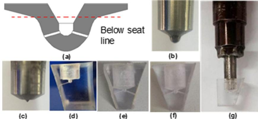
Fig. 2. Common-rail injector nozzle and real-size optical nozzle tip: (a) the incised position, (b) original injector nozzle, (c) cut injector nozzle without nozzle tip, (d) & (e) & (f) transparent nozzle tip and (g) the assembled injector nozzle.
