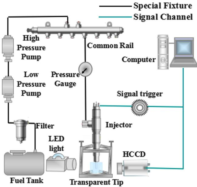
Fig. 1. Schematic of the experimental visualization system for internal nozzle flow and spray.
