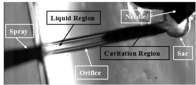
Fig. 3. The typical image of cavitating flow inside the tested nozzle.
