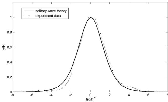
Fig. 1. Comparison of free surface profile between the solitary wave gauge measurement and the theoretical equation results.
