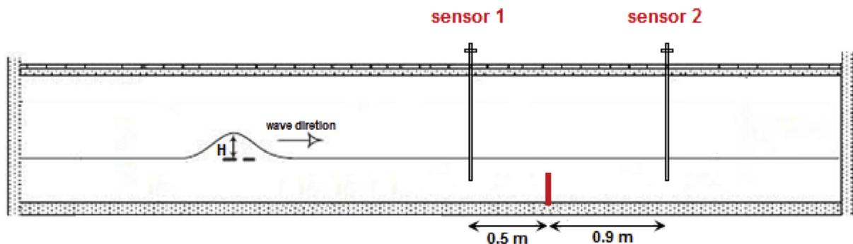
Fig. 2. Schematic diagram of the location of wave height gages.
