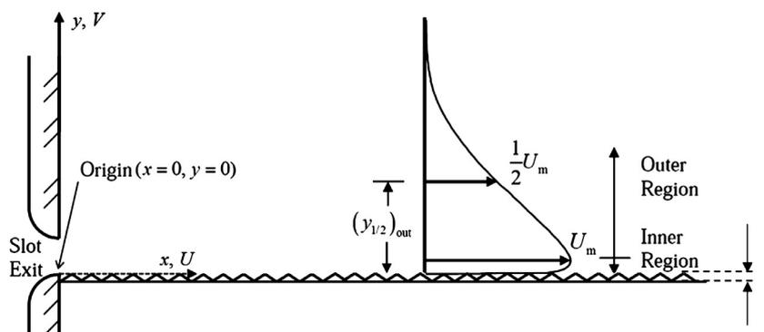
Fig. 1. Schematic representation of a plane turbulent wall jet on a rough surface.
