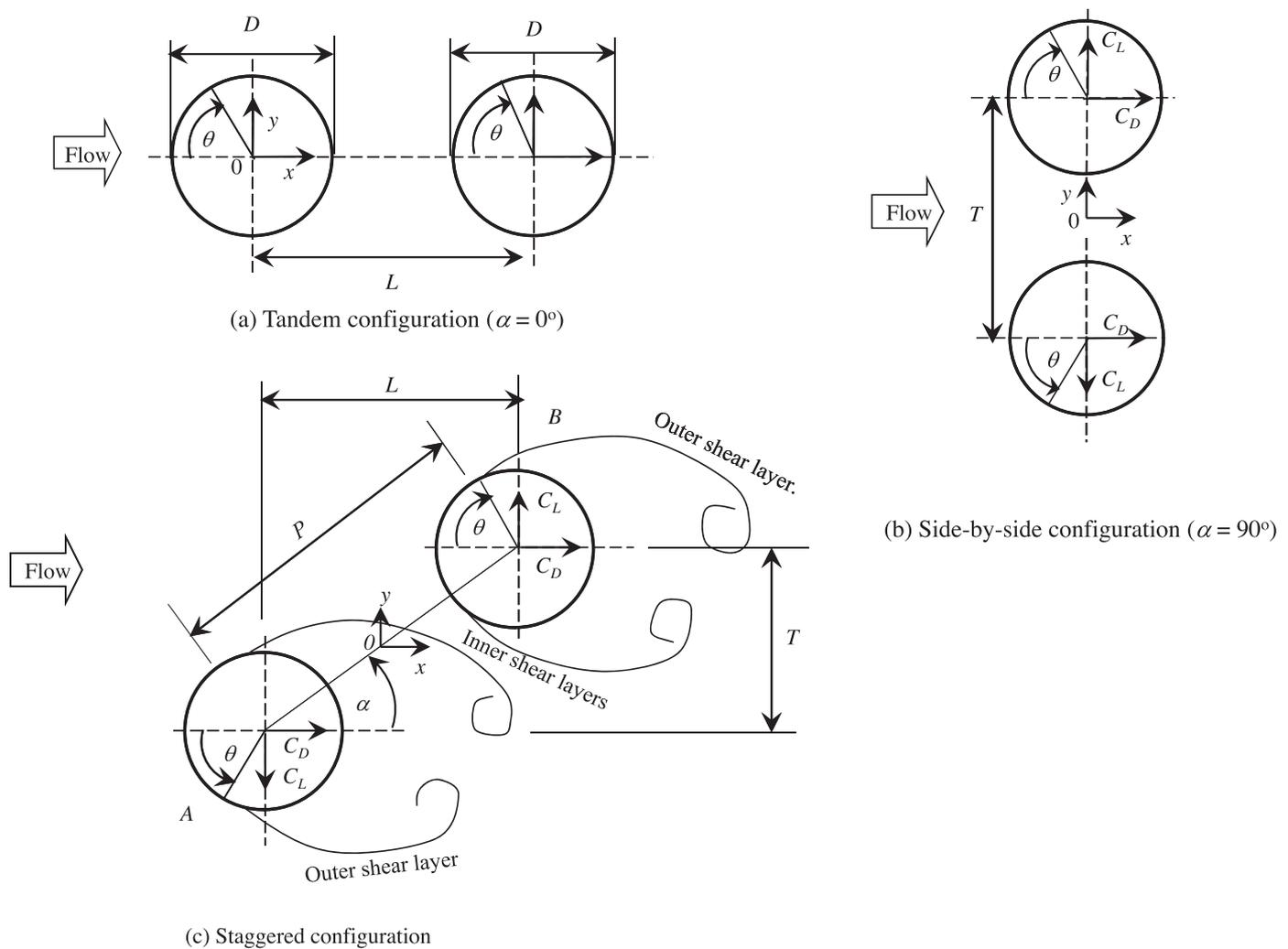
**Fig. 1.** Arrangements of cylinders and definitions of symbols.  $D$ : cylinder diameter;  $P$ : cylinder center-to-center spacing;  $x, y$ : Cartesian coordinate;  $L$  and  $T$ : streamwise and transverse separations between the cylinders, respectively;  $\alpha$ : stagger angle;  $\theta$ : azimuthal angle;  $C_D$  and  $C_L$ : time-mean drag and lift, respectively.
