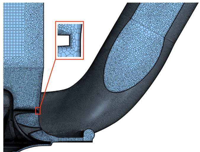
Fig. 2. Slice of computational grid, showing a close-up of tip clearance and the boundary layer mesh inflation. Inlet and outlet ducts present the displayed grid pattern until their respective boundary.
