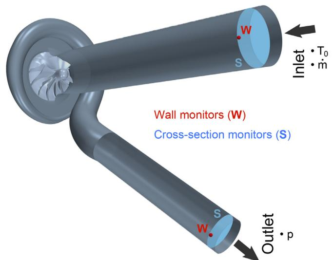
Fig. 1. CFD domain including monitor types and locations and flow variables imposed at the boundary conditions.
