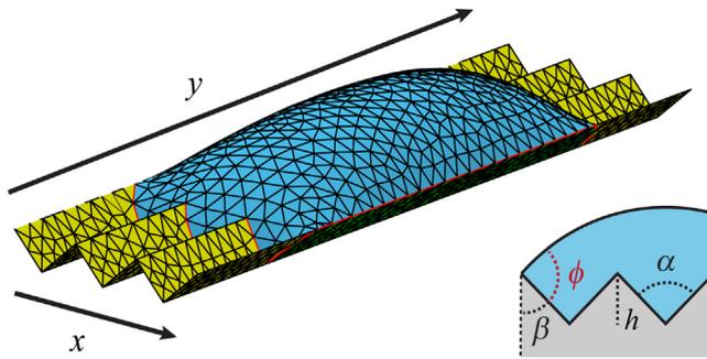
**Fig. 1.** The droplet equilibrated at pinning angle  $\phi$  deposited on a series of triangular grooves of dihedral angle  $\alpha = 90^\circ$  and height  $h = 0.1$  ( $\tilde{V} = 400$ ,  $\theta_Y = 75^\circ$ ,  $G = 3$ ). The opening angle  $\beta$  at the extreme edge is also shown.
