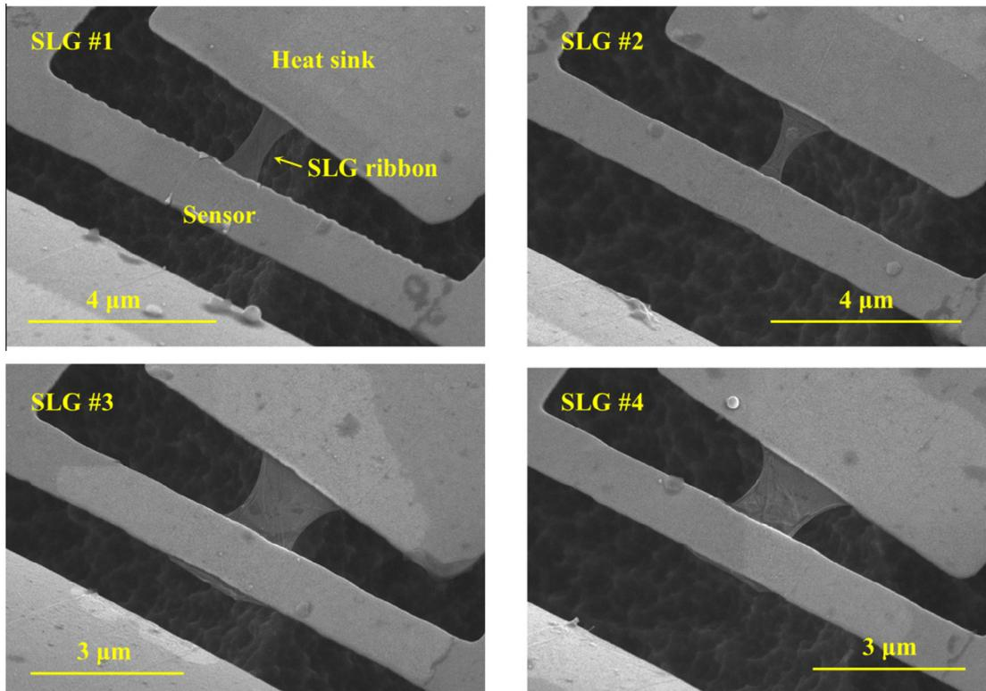
Fig. 1. SEM images of four SLG samples. Samples #1 and #2 are narrow ribbons, whose widths are 0.85 μm and 1.22 μm, respectively. Samples #3 and #4 are wide ribbons, whose widths are 1.92 μm and 2.08 μm, respectively. The SLG sample is suspended between a micro-beam sensor and heat sink pad. The sensor serves as both Joule heater and precise resistance thermometer.
