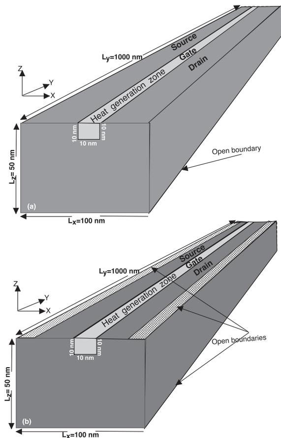
Fig. 1. (a) Case one: the 3-D silicon structure with bottom open boundary condition. (b) Case two: the 3-D transistor with two top and one bottom open boundaries. All other boundaries are adiabatic for both cases.
