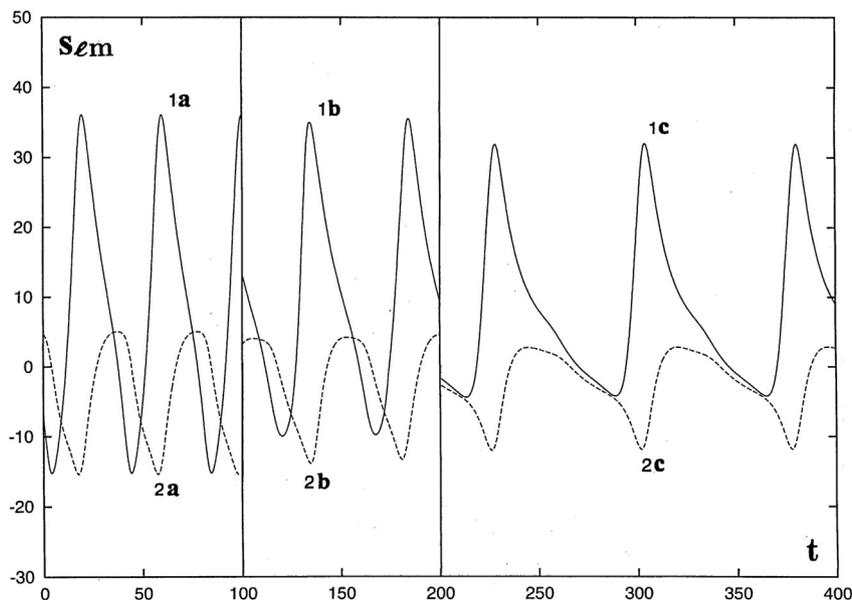
Fig. 2. Dependences of  $S_{l,m}$  on time ( $m = 1, 2$ ) at  $Q_T = 0$  (lines 1a, 2a);  $-0.75$  (lines 1b, 2b);  $-1.35$  (lines 1c, 2c);  $G = 112.5$ ;  $K = 0.025$ ;  $\epsilon = 0.01$ ;  $G_Q = -25$ ;  $L = 2.74$ ;  $a = 1$ .
