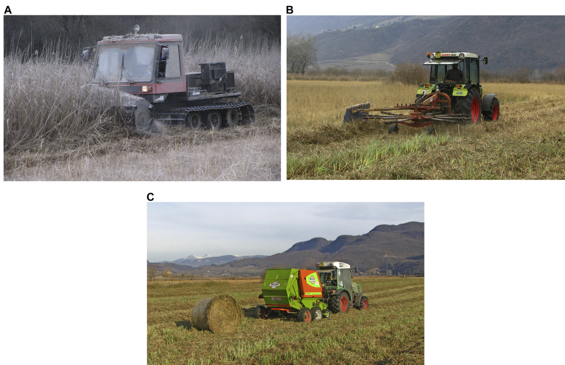
Fig. 1. The reed collection system on trial: chopping (top left), windrowing (top right) and baling (bottom).
