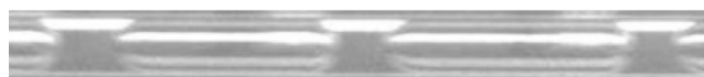
Fig. 2. Visualization of slug flow in a 1.7 mm diameter single horizontal mini tube [5].
