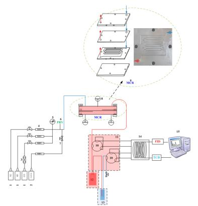
Fischer-Tropsch (FT) synthesis was carried out in a microchannel reactor under a wide range of operating conditions using mesoporous supported bimetallic Co-Ni catalyst for process intensification. The response surface methodology (RSM) and central composite design (CCD) were employed in determining the optimal condition for light olefin production.  $\Box$ New
