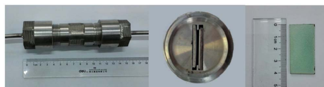
Fig. 1. Scheme of micro-channel reactor and catalyst plate in SMR reaction.
