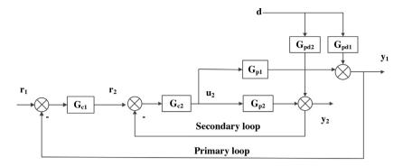
Fig. 1. General block diagram of parallel cascade control structure.
