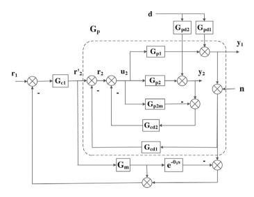
Fig. 2. Proposed Smith predictor based parallel cascade control structure.
