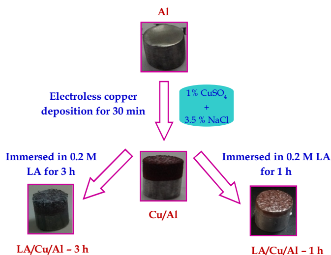
Fig. 1. Schematic representation of electroless copper deposition (30 min) and laurylamine assembly (1 h and 3 h) over Al surface respectively.
