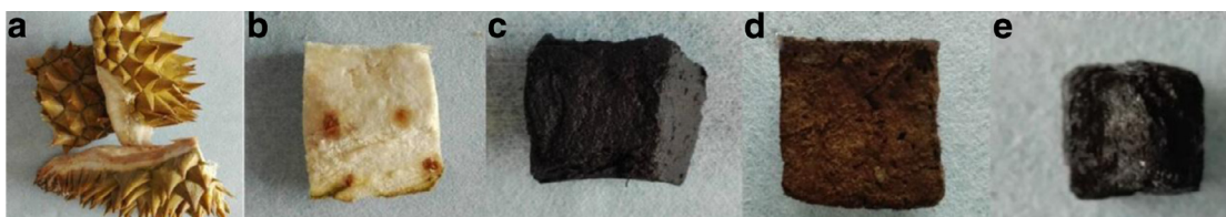
Fig. 1. The photographs of raw material (a and b), hydrogel (c), aerogel (d), and carbon aerogel (e) in the preparation process of DSCA.
