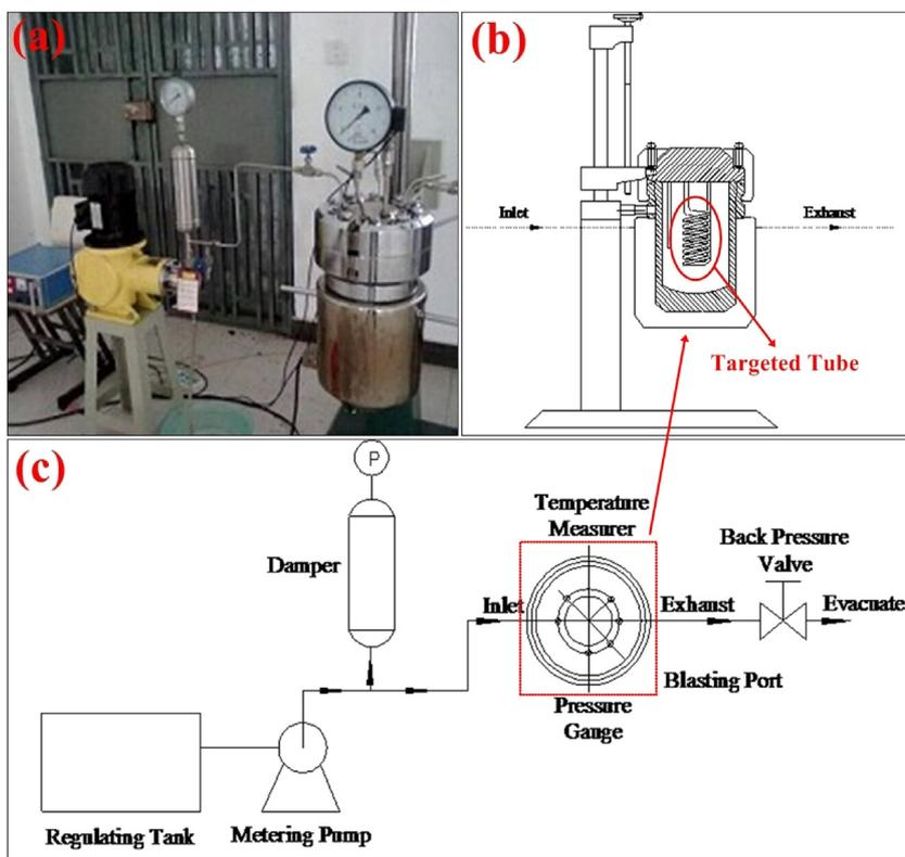
Fig. 1. Figures of the lab-scale test reactor system: (a) picture of the reactor, (b) structure diagram of the reactor, (c) structure diagram of reactor system.
