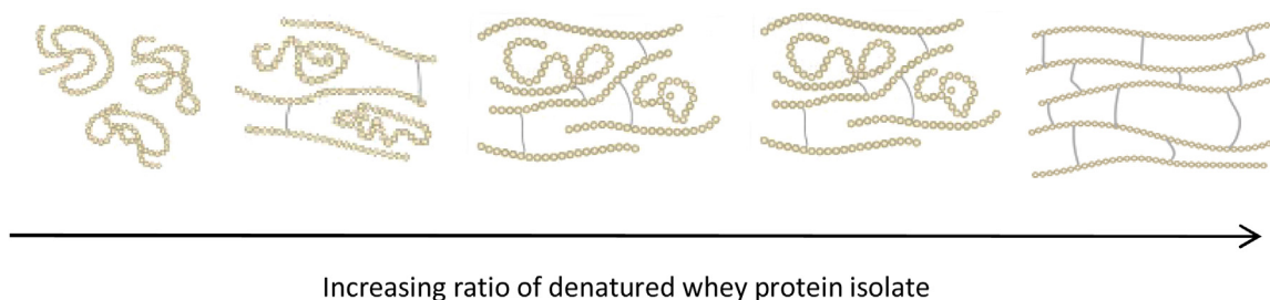
Fig. 1. Schematic illustration of protein unfolding and linearization by heat treatment and formation of disulfide bonds between the exposed cysteine units with increasing degree of denaturation.
