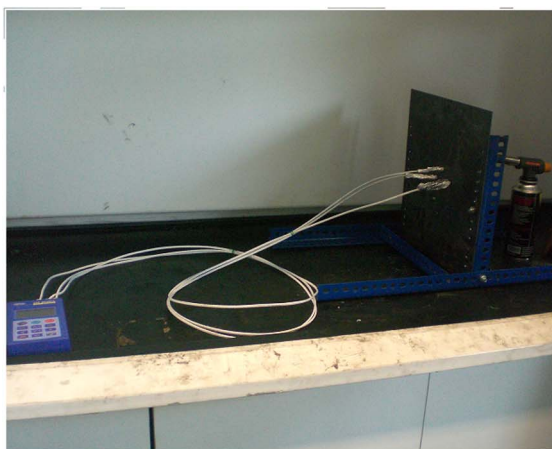
Fig. 1. Fire test setup for the heat insulation test of the intumescent formulation: (a) portable Bunsen burner, (b) stand, and (c) sample of intumescent coating [15].
