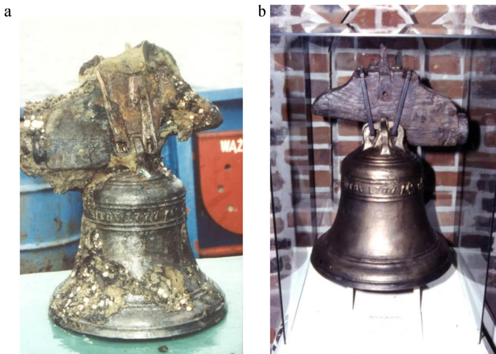
Fig. 1. The bell from General Carlton: (a) before and (b) after cleaning.
