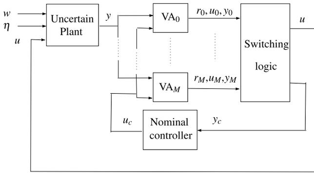
**Fig. 1.** Proposed FTC scheme with uncertain plant, bank of virtual actuators  $VA_0$  to  $VA_M$ , switching logic and nominal controller.
