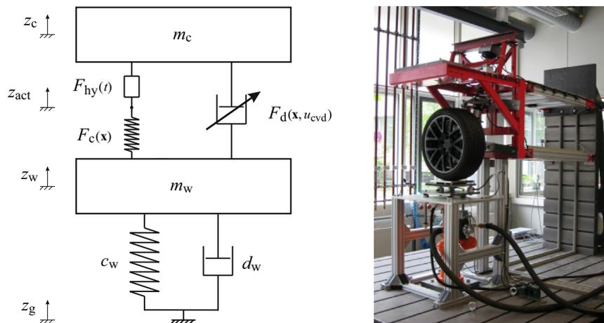
Fig. 1. Model (left) and test rig (right) of hybrid quarter-car configuration.
