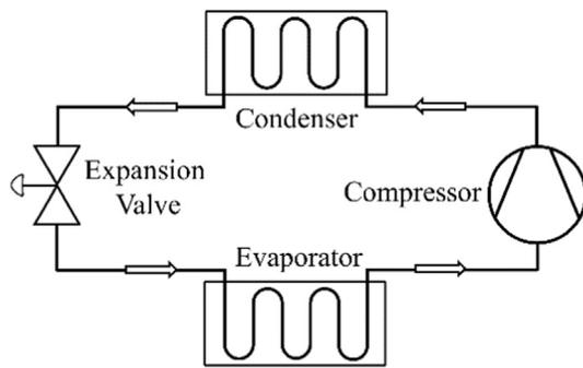
Fig. 1. Schematic of a basic vapor compression system.
