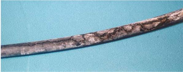
Fig. 2. Surface tracked covered conductor [12].
