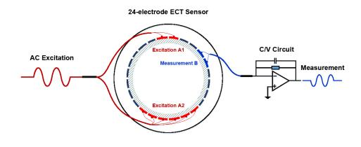
Keywords: Electrical Capacitance Tomography; multi-electrode sensing; simutaneous asymetric excitation; image reconstruction
