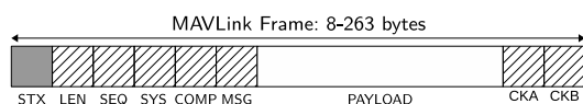
Fig. 1. Example of a MAVLink packet. Each field has 1 byte length, except the payload field that can assume a variable length. The payload field is optional
