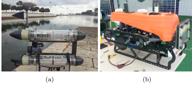
Figure 2. The autonomous vehicles: (a) the MEDUSA-class as the surface and (b) BUDDY as the underwater agent
