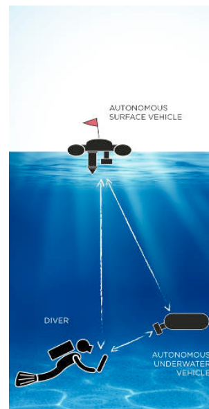
Figure 1. The CADDY concept - a diver with an underwater agents as a slave and diver monitoring platform and a surface vehicle as a communication and absolute navigation relay for underwater agents.
