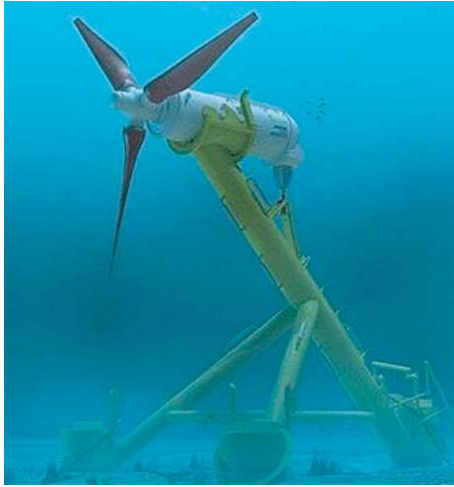
Fig. 1. TEC based on open rotor configuration for marine current harnessing (Andritz (2016)).
