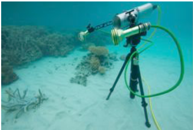
Fig. 1. An analog prototype of UHI at 5 m depth on Lizard Island, Great Barrier Reef, Australia, January 2011. The underwater tripod was equipped with a panorama scanning unit and two 35W halogen lamps (battery powered) for scanning of different colour groups of soft- and hard coral species.
