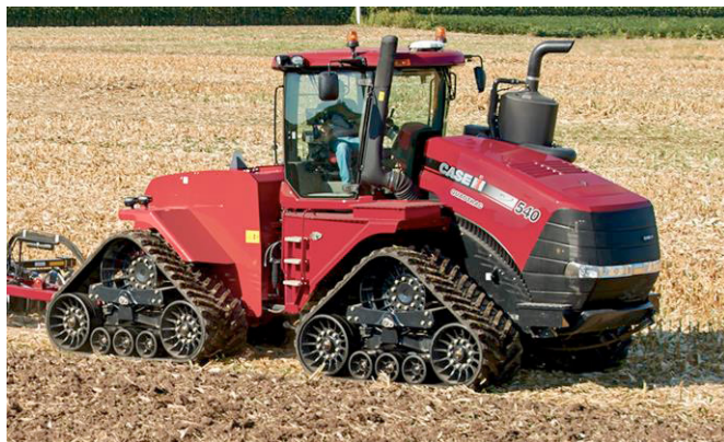
Fig. 1 Case IH Steiger with articulated frame-steering (Case IH)
