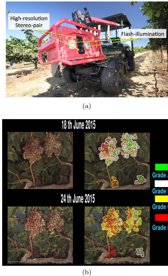
Fig. 1. An overview of the Yield Mapping System (a) Imaging Unit in Vineyard – consisting of stereo cameras and a pair of flashes for capturing high resolution images. (b) Left: Raw images of clusters on the 18 th and 24 th June 2015. Right: Image automatically processed to detect clusters and evaluate color development. Berries that are well-colored are highlighted by a red square. Clusters classified as having sufficient level of well-colored berries are highlighted with red contour. Those berries and clusters that are deemed not well colored are highlighted yellow.
