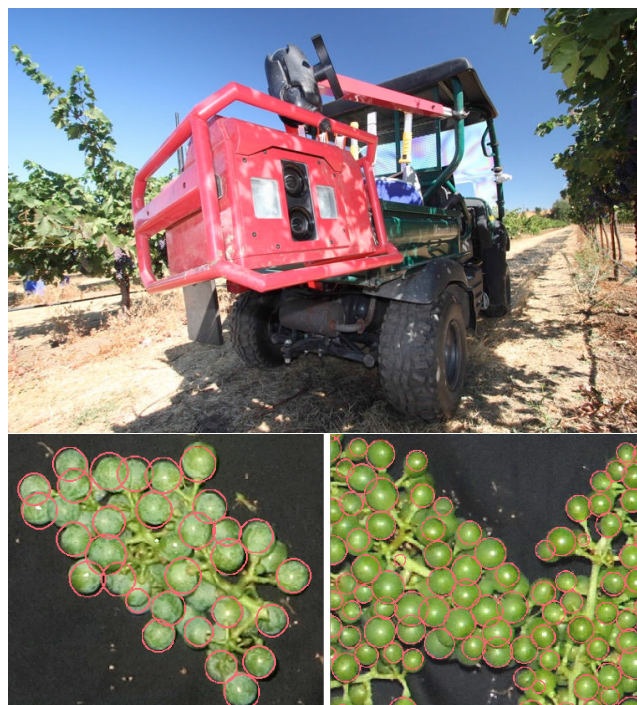
Fig. 1. Vehicle mounted imaging system (top) and sample images of estimated grape diameters for Cabernet Sauvignon (bottom-left) and Petite Syrah (bottom-right)
