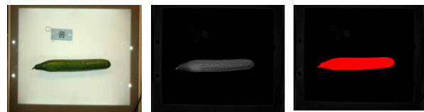
Fig. 3. Separate cucumber segmentation: RGB image (left), excessive green image (middle) and the final cucumber segmentation produced by the excessive green image thresholding (right).
