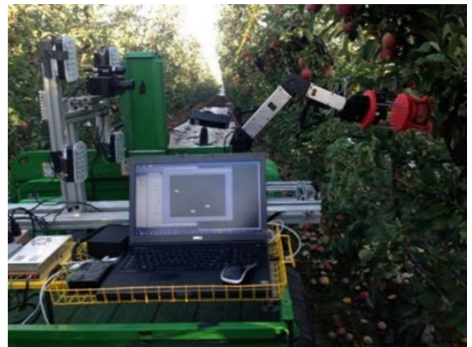
Fig.1. Field evaluation of a robotic apple harvester (Silwal, et al., 2016).
