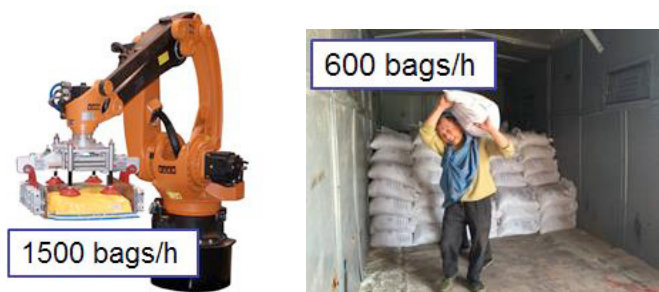
Fig.1. Comparison of the efficiency between the handling robot and manual method during loading and unloading
