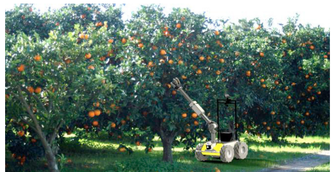
Fig. 1: An illustration of the re-configurability concept to use on a peach harvesting task (top) using a PRR arm, and on a tangerine harvesting task (bottom), using a RRP arm.
