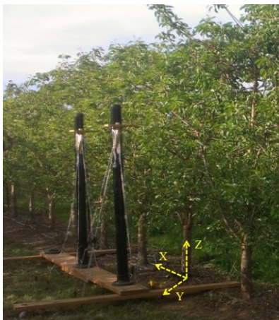
Fig. 1. A wooden frame carried six digitizer ‘source’ modules, in order to cover the volume of large trees.
